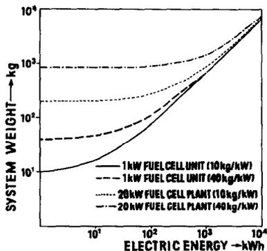
Fig. 4. System weight and electric energy for a complete  $H_2-O_2$  fuel cell power plant with reactants stored as liquids.
