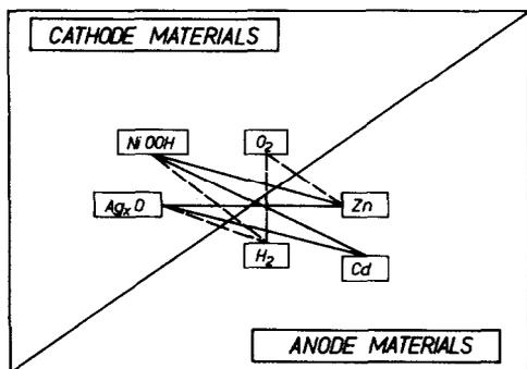
Fig. 1. Cathode and anode materials for first and second generation secondary spacecraft batteries.
