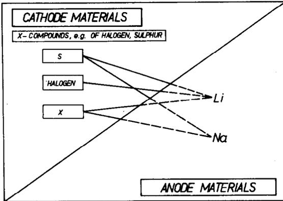
Fig. 2. Cathode and anode materials for third generation secondary spacecraft batteries.
