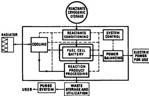
Fig. 3. Subsystems for an H<sub>2</sub>-O<sub>2</sub> fuel cell power plant.
